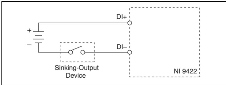
**Figure 3.** Connecting a Sinking-Output Device to the NI 9422
