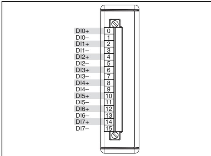
**Figure 2.** NI 9422 Terminal Assignments
