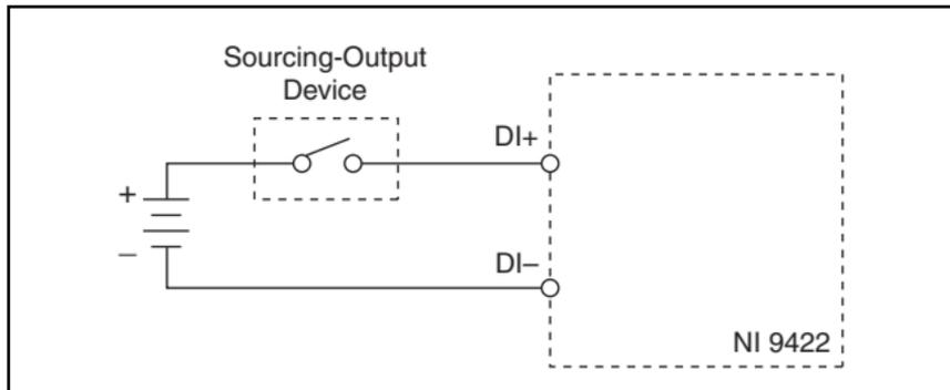
**Figure 4.** Connecting a Sourcing-Output Device to the NI 9422
